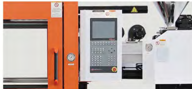
Advanced intelligent controller system with 10.4" display MPC 7.0 intelligent networkable computer controller, designed in Japan
