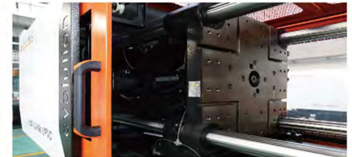
Extra-wide doors and guards Perfect for UPVC pipe fittings 160-200T - 300mm 260-480T - 500mm 560-650T - 700mm
