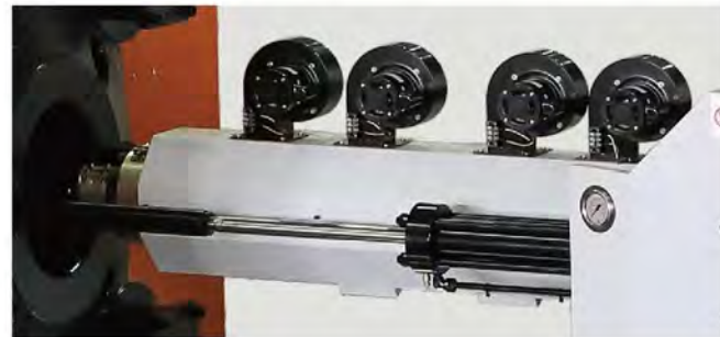
Fan-cooled barrel Convection-type cooling tunnel design, high efficiency, high temperature stability.
