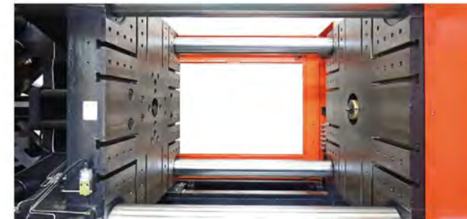
T-slots plus mounting holes Best of both worlds, no need to choose
