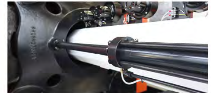
Dual balanced injection cylinders Smooth injection movements
